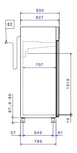
= Drain = Electri Electrical inlet (power)
